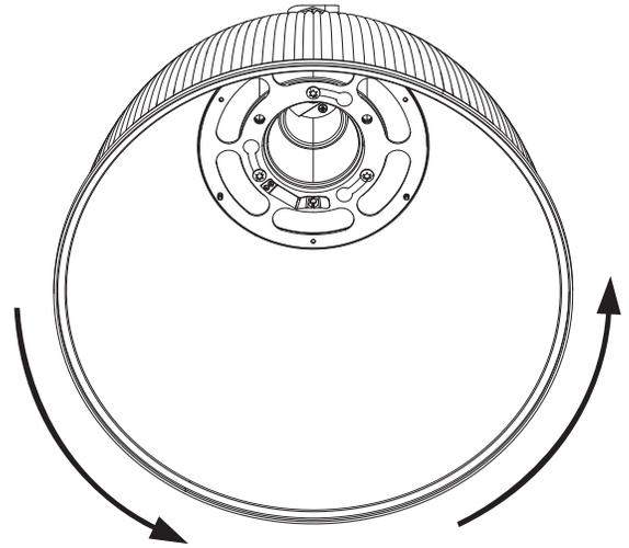
Twist and lock reflector. The spring pin will lock into the base reflector.
