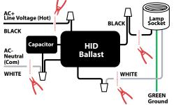
6. Connect Hot (100VAC-277VAC) to black wire and Neutral to white wire connected to socket.
